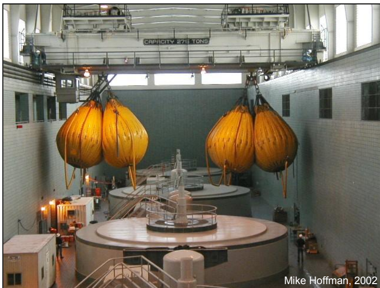
Figure 12. Crane being tested at a Tennessee Valley Authority powerplant using water weight bags™ (photo by Mike Hoffman; photo courtesy of Jim Jota, Imes, Inc., 2002).
