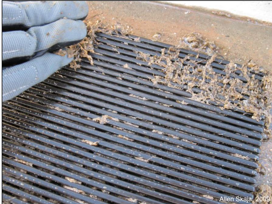
Figure B-14. This is an example of a foul release coating that has been in the water for 18 months. Mussels and algae growth may attach to the surface under certain flow rates; however, they are easily removed (photo courtesy of Allen Skaja, 2009).
